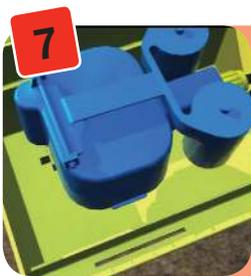
Once you have connected the AQUAvalve to the 6mm pipe, simply pull the pipe back through so that all the excess pipe inside the AQUAbox Straight is pulled out. As you pull the pipe out lower the AQUAvalve so that it locates onto the Tee section in the AQUAbox Straight.
